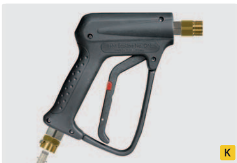
Professionelle Pistole R+M EcoLine No. ONE. Max. 250 bar / 45 l/min / 150 °C
