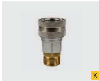
Kupplung : AG. Messing vernickelt + Messing. Max. 250 bar / 150 °C
