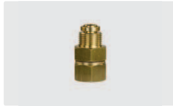
3/8" AG : 3/8" IG. Messing. Max. 220 bar / 90 °C
