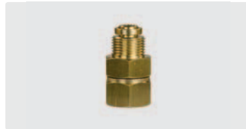
3/8" AG : 1/4" IG. Messing. Max. 220 bar / 90 °C
